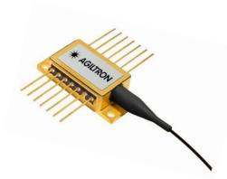
The 1440nm series laser diodes are fabricated in a hermetically sealed 14-pin butterfly package. The laser diodes contain a monitor photodiode, thermoelectric cooler (TEC), and a thermistor to secure high-quality laser performance. Our laser products are Telcordia GR-468 qualified and in compliance with RoHS Directives.
